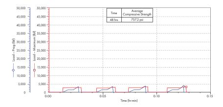
Within the density range of 9.0 to 10 lbm/gal, the high ultimate compressive strength of CircuLite CS-featherweight cement makes the system ideal as a primary slurry for various applications.
