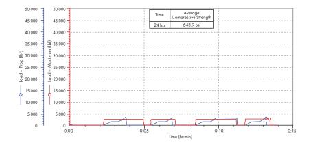
At 9.0 lbm/gal, the early compressive strength development of CircuLite CS-featherweight cement is unsurpassed by that of any other cement system at the same density.
