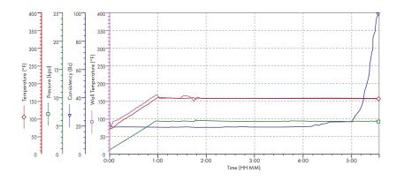
CircuLite CS-featherweight cement slurry can be customized to deliver high performance between 80 to 160°F and ranging in density from 9.0 to 10 lbm/gal.
